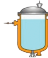
Jacket heat exchanger
